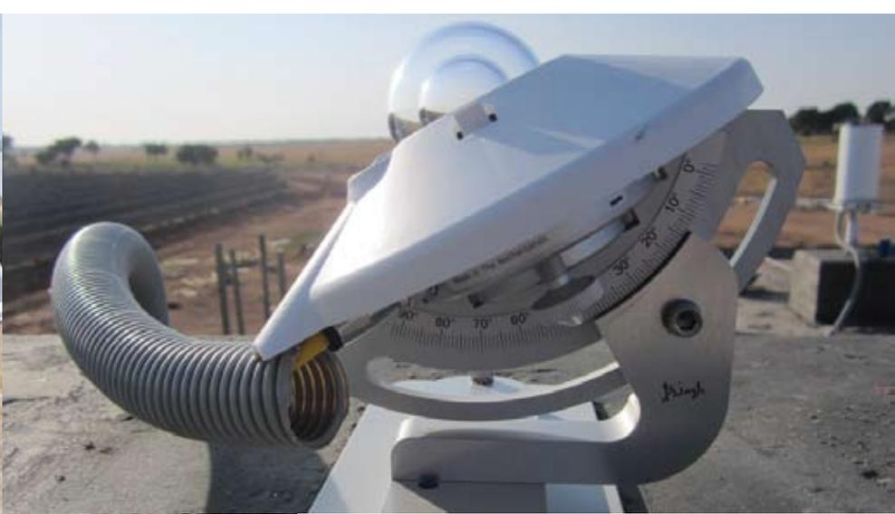
from real world field conditions, additional measurements using pyranometers and/or reference cells are required to monitor PV performance.
